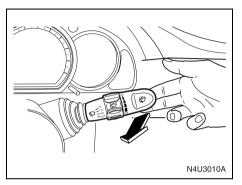
To wash your windshield, pull the windshield wiper/washer lever toward you with the ignition in the ON position.
